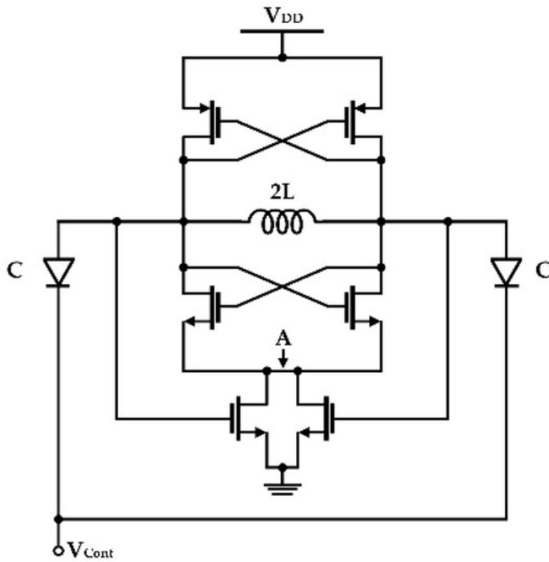
**Figure 2.** Schematic of a CMOS LC-VCO with the switched-biasing technique to the current source (reproduced with permission from the author, RF CMOS low-phase-noise LC oscillator through memory reduction tail transistor; published by IEEE, 2004)<sup>[34]</sup>.
