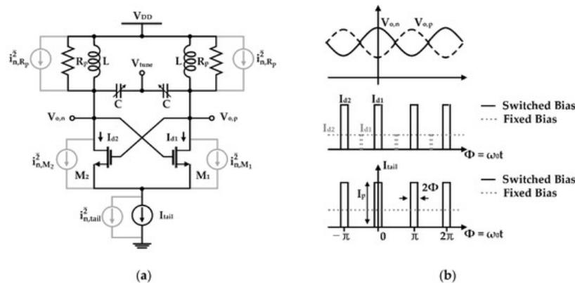
**Figure 3.** Analysis of VCO characteristics depending on the pulse modulation of the current source using the impulse sensitivity function theory: (a) schematic of the differential LC-VCO; (b) conceptual waveforms of the output voltages and drain currents of the VCO and the bias current by the pulse-modulated current source (reproduced with permission from the author, Tail current-shaping to improve phase noise in LC voltage-controlled oscillators; published by IEEE, 2006)<sup>[47]</sup>.
