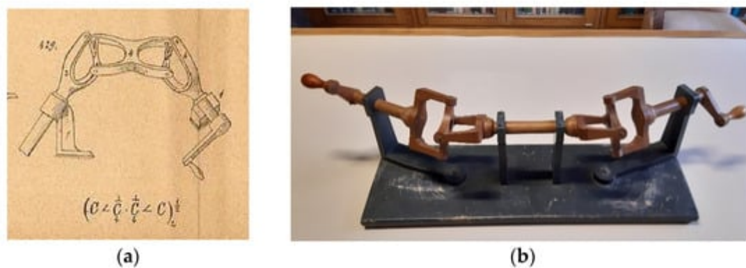
Figure 2. A model of the double Hooke's joint: (a) in the treatise of Masi [16] ; (b) the corresponding wooden model at the University of Bologna.
