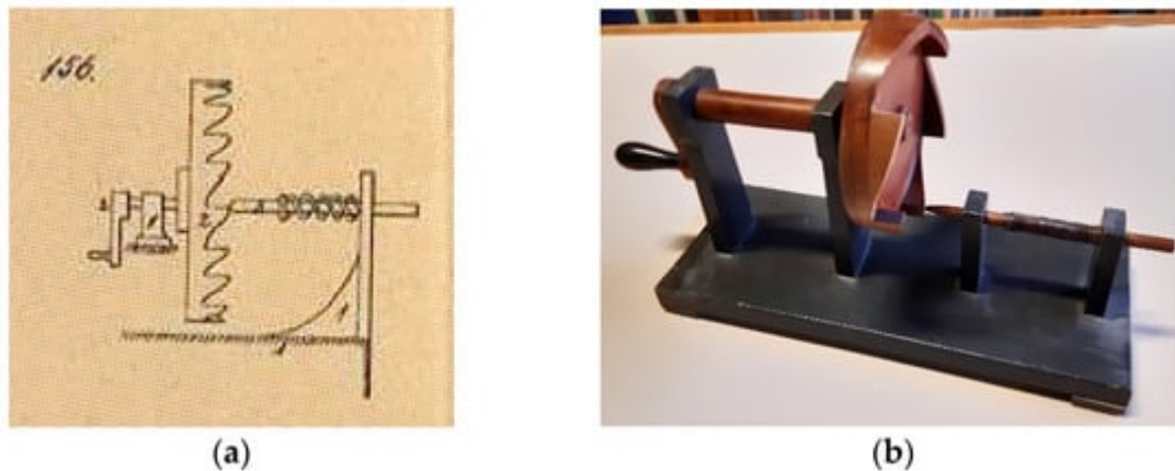
Figure 1. A model of cylindrical cam disk: (a) in the treatise of Masi [15] ; (b) the corresponding wooden model at the University of Bologna.
