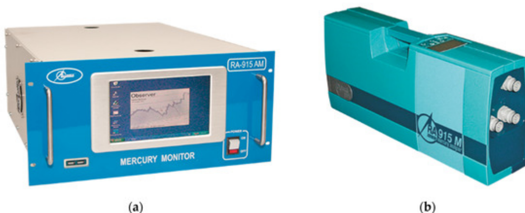
Figure 2. Measurement technique: (a) The RA-915AM air mercury monitor; (b) The RA-915M portable mercury analyzer.
