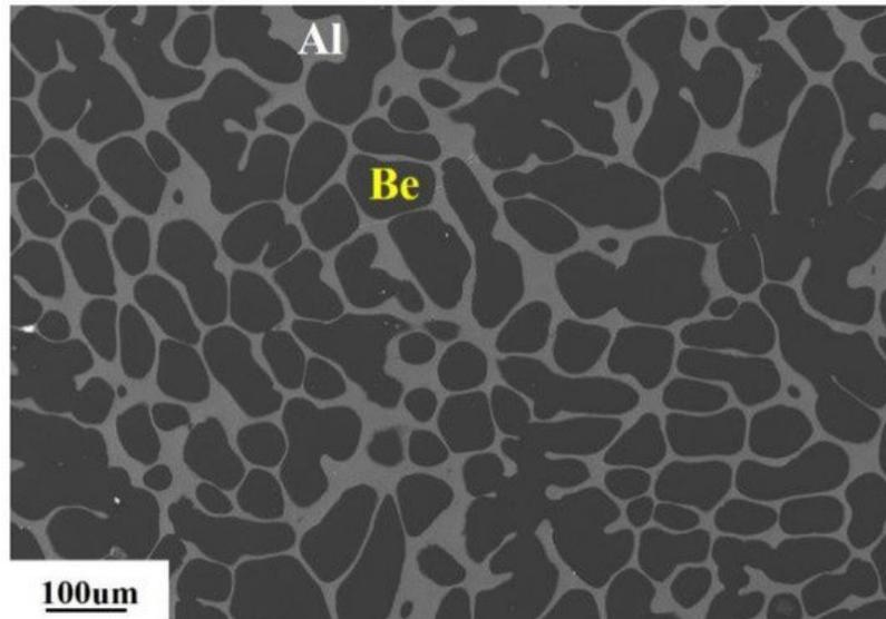
**Figure 2.** The SEM image of Be-Al alloy.
