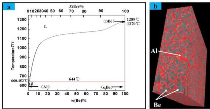
**Figure 1.** The phase diagram of Be-Al alloy (a), three-dimensional microstructure (b) [1]. Reprinted/adapted with permission from Ref. [1]. Copyright 1994, Elsevier Ltd.
