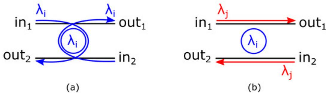
**Figure 3.** A  $2 \times 2$  PSE supports (a) two on-resonance signals and (b) two off-resonance signals.
