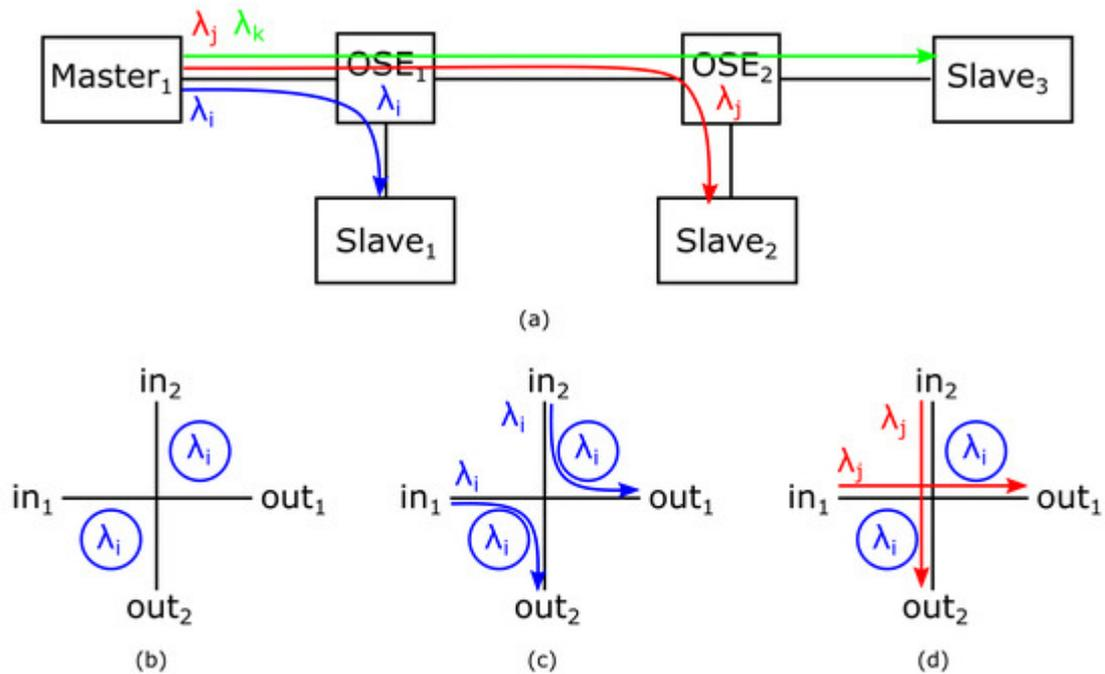
**Figure 1.** (a) A simple WRONoC topology. (b) A  $2 \times 2$  CSE structure. (c) On-resonance signals change their propagation directions. (d) Off-resonance signals pass through the CSE without direction change.
