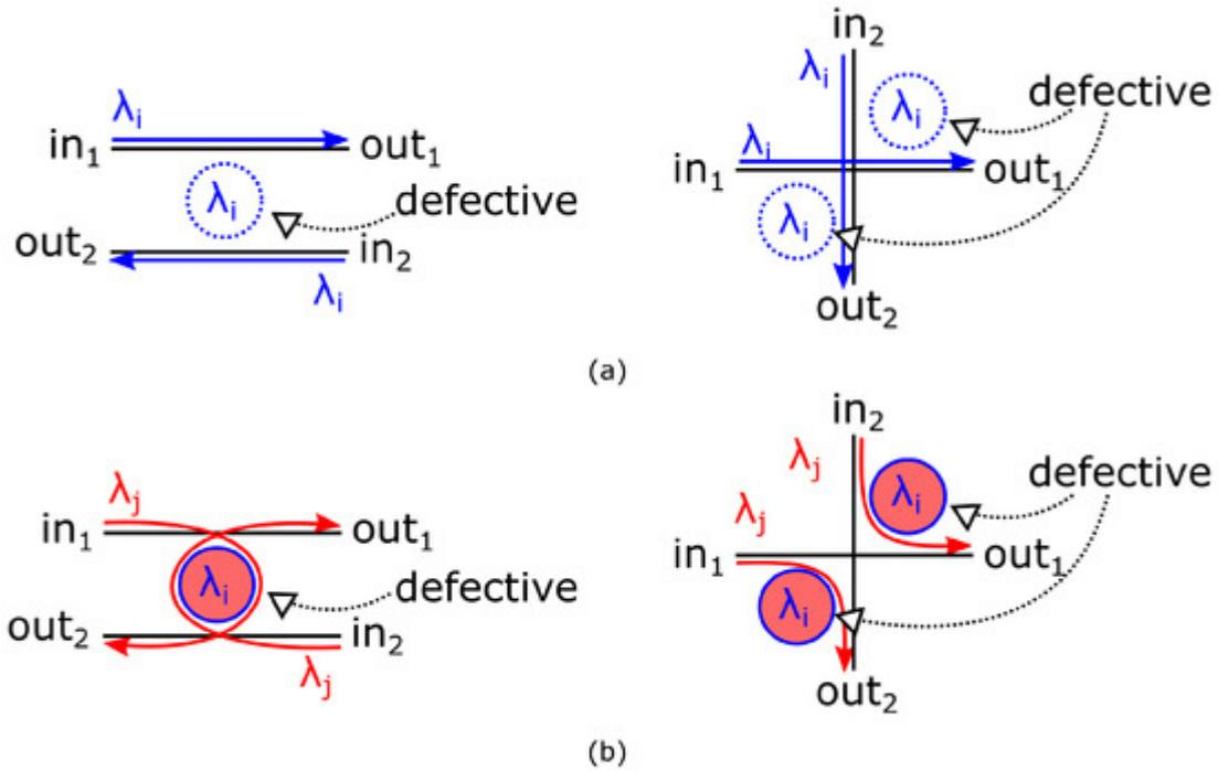
Figure 5. (a) The s-a-0 signal fault. (b) The s-a-1 signal fault.
