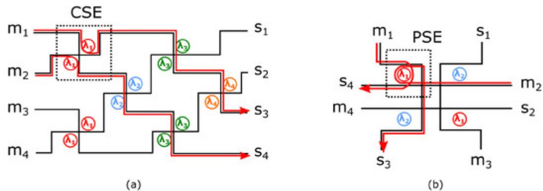
Figure 6. (a) A  $4 \times 4 \times 4$   $\lambda$ -router. (b) A  $4 \times 4 \times 4$  Hash.
