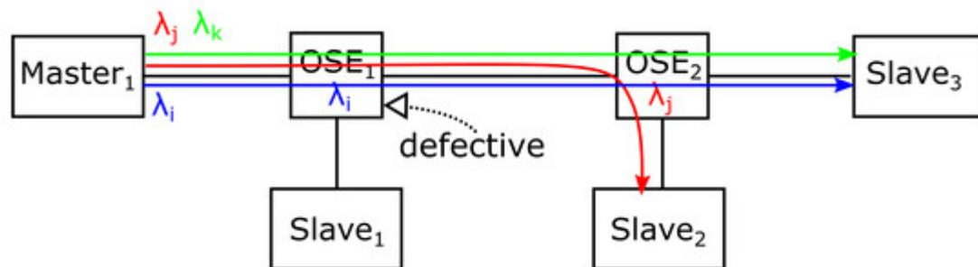
**Figure 2.** The MRR in OSE<sub>1</sub> is defective and the signal on  $\lambda_i$  fails to be coupled to the MRR.
