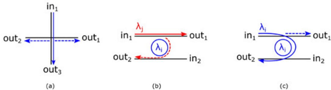
**Figure 4.** The first-order noise is generated (a) when a signal passes a waveguide crossing, (b) when a signal passes an off-resonance MRR, and (c) when a signal is on-resonance with an MRR.
