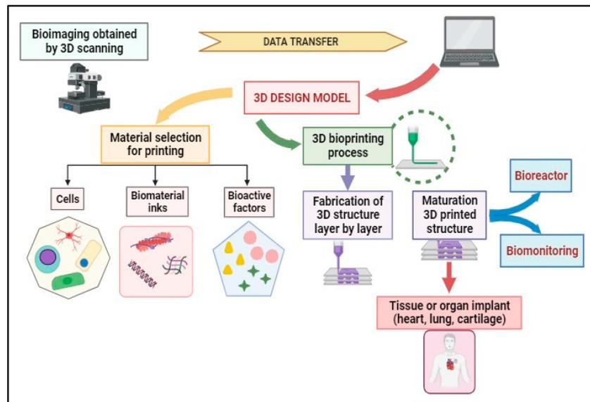
**Figure 4.** 3D bioprinting process flow.
