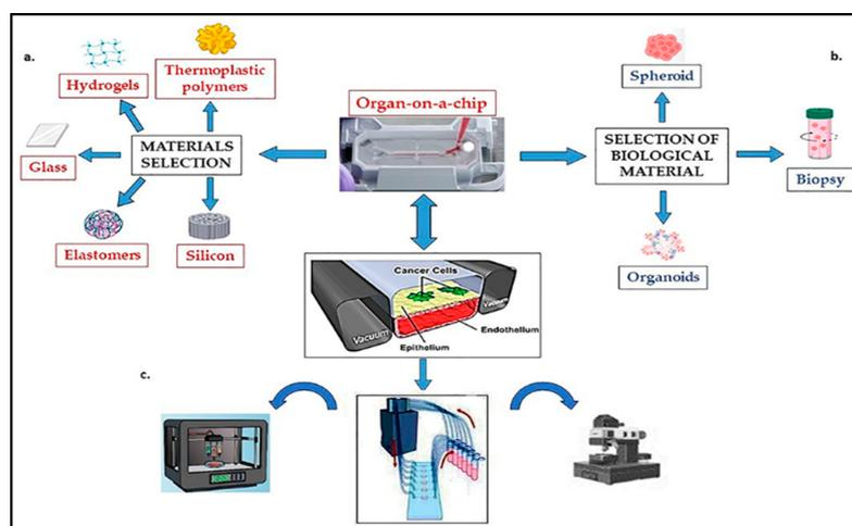
**Figure 6.** Components of functional tumor-on-a-chip system: (a) material selection and microchip fabrication; (b) selection of biological material; (c) peripheral equipment (Incubators, Pumps for perfusion, Mechanical stimulation, Controls and sensors, Microscope).
