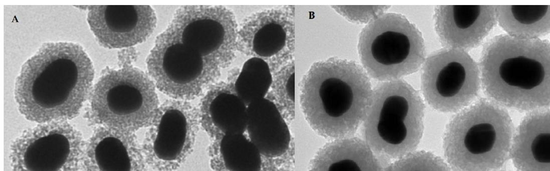
Figure 5. Representative image of PET-SERRS nanoparticles with non-optimized <sup>68</sup>Ga-labeling (A) with visible degradation of silica shells and after the optimization (B) with improved stability of the silica shells [29].
