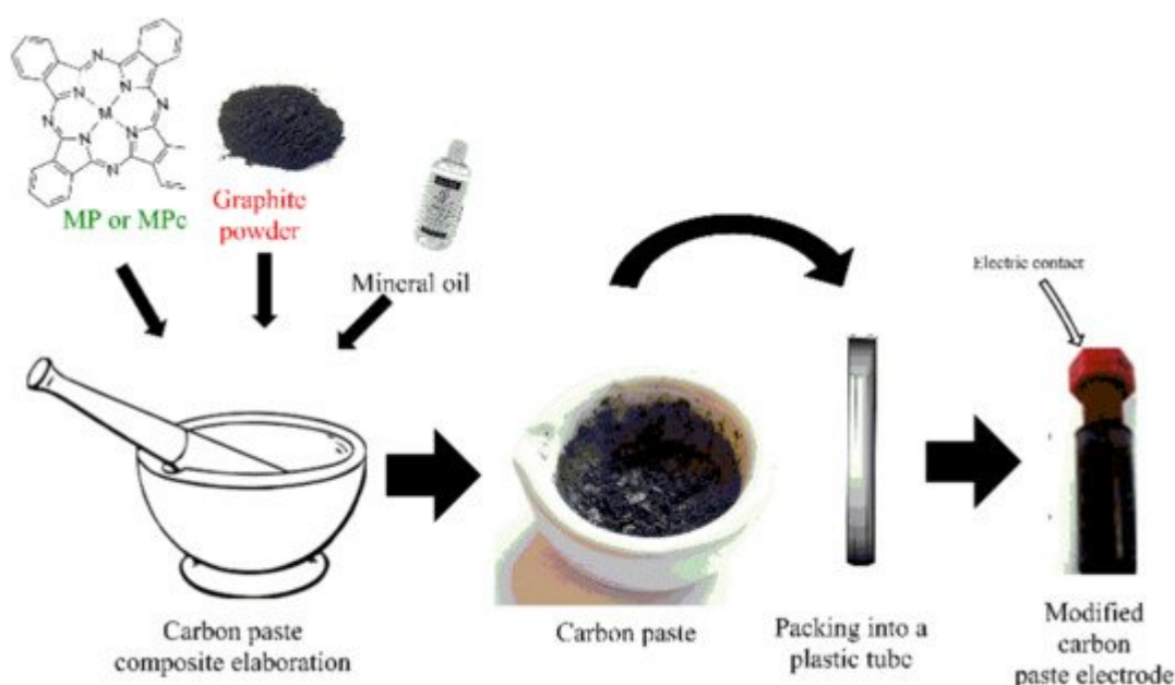
Figure 3. A simple modified CPE's elaboration process.
