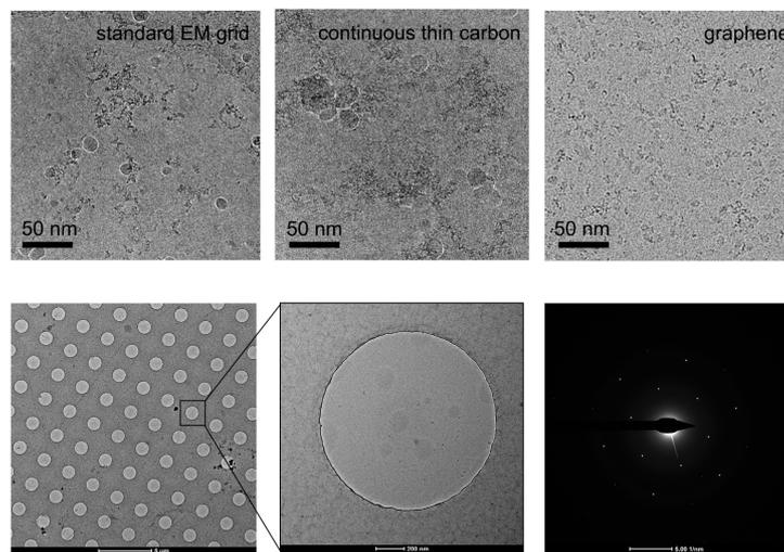
**Figure 4.** Improvement of graphene grid on the protein distribution by preventing from adsorption to the AWI. The graphene grid examined in the diffraction mode before sample preparation showed single-layer coverage.
