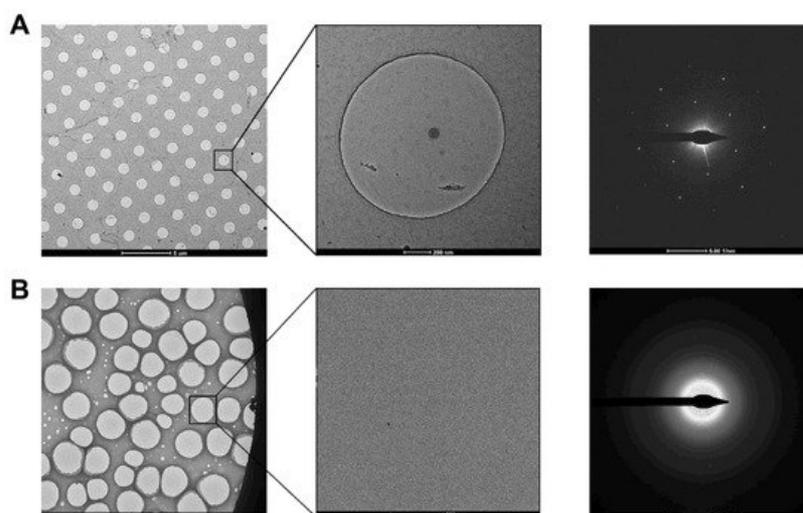
**Figure 3.** Examination of graphene and GO grids in the diffraction mode. (A) Graphene grid prepared using Quantifoil grid. The diffraction pattern showed the single-layer coverage in the zoomed-in hole. (B) GO grid prepared using holey carbon grid (purchased from Beijing Zhongjingkeyi Technology Co., Ltd. Beijing, China). The diffraction pattern showed the multi-layer coverage in the zoomed-in hole.
