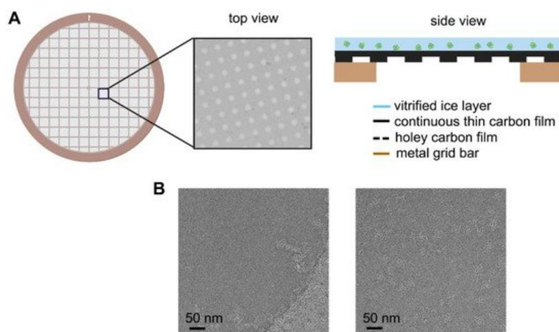
**Figure 1.** Schematic diagram of improved EM grid and its improvement on the particle distribution. (A) Commonly used arrayed EM grid covered with additional layer of continuous thin carbon film on the holey carbon film. (B) Example of ryanodine receptor 1 (RyR1) distribution in the vitrified ice without (left panel) and with (right panel) continuous thin carbon film spanning on the hole.
