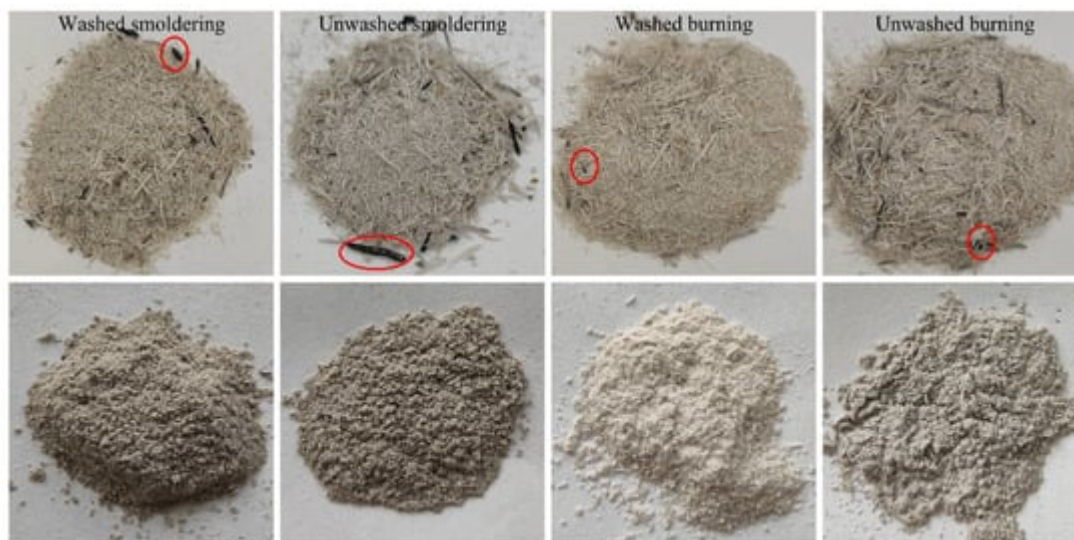
Figure 3. Photos of four types of rice husk ash (circles show black particles in ash).
