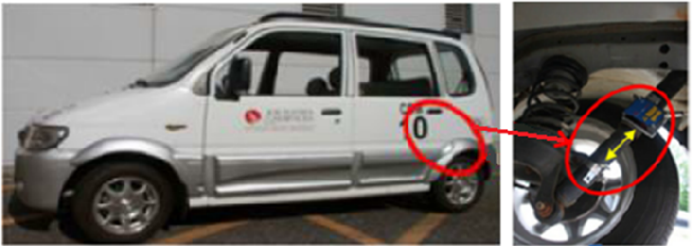
Figure 11. Location of the shock absorber to collect energy in the minivan vehicle [59].
