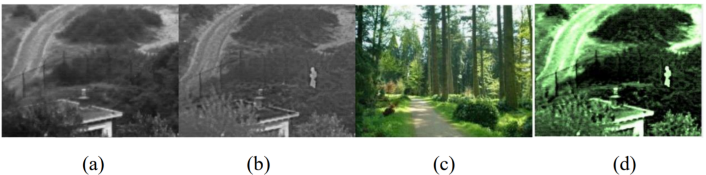
Figure 1. Example of infrared and visible image fusion for color vision at night. (a) visible light images; (b) infrared images; (c) reference images; (d) fusion of images.
