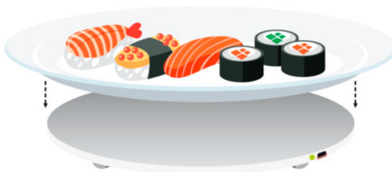
Figure 4. A custom-made electronic scale that is connected via bluetooth with a smartphone application measuring the reduction of the food placed on the scale along with self-recording of hunger and fullness [8].
