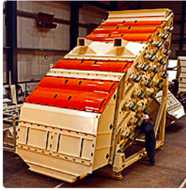
Sizer 2000 for screening coarse to small particles. https://handwiki.org/wiki/index.php?curid=1148271
