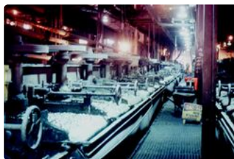
Froth flotation cells used to concentrate copper and nickel sulfide minerals, Falconbridge, Ontario.
