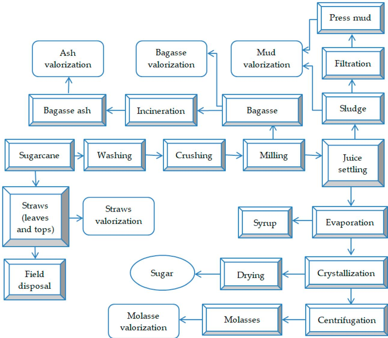
**Figure 1.** Sustainable technological flow of cane sugar production, highlighting the generated waste and by-products.
