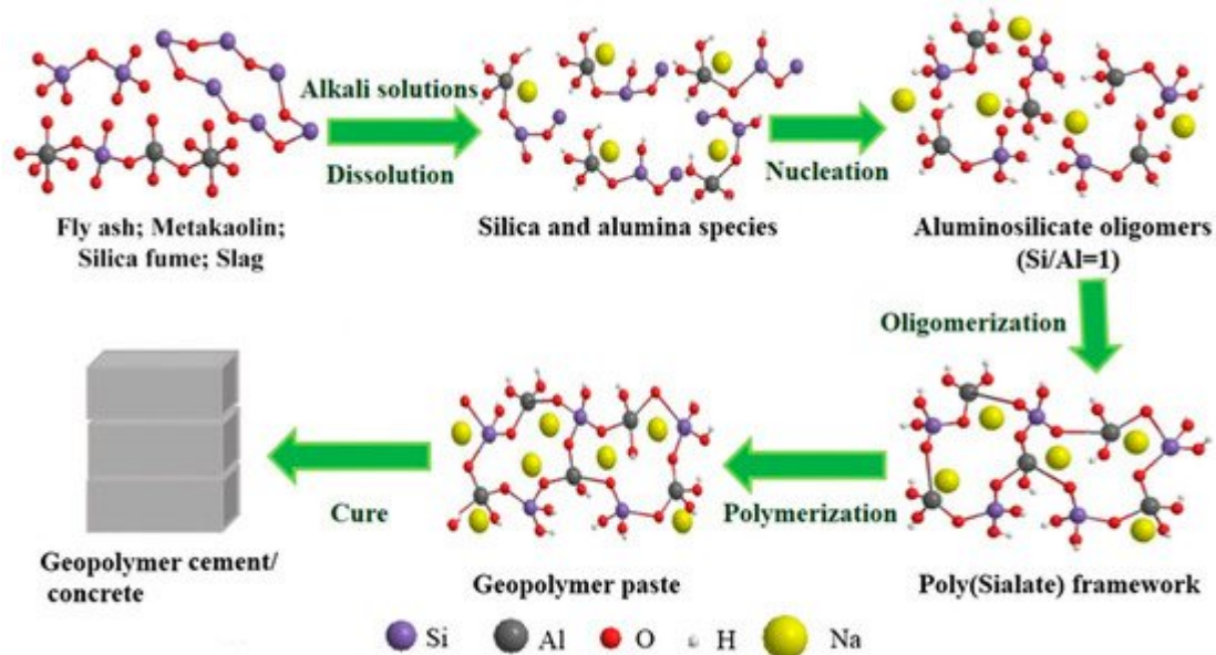
Figure 1. Geopolymerisation process for the fabrication of geopolymer cement/concrete. Different sources of siliceous and aluminous materials are used for the production of geopolymers, the most common including fly ash, metakaolin, silica fume, ground granulate blast slag, and other ashes such as volcanic and biomass ashes. Reprinted with permission from ref. [9]. Copyright 2016 Elsevier.
