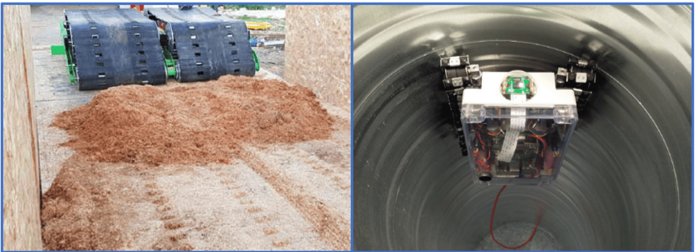
Figure 6. TGMR-CT with flat tracks for flax raw material compacting ( left ); TGMR for pipe inspection with magnetic locomotion ( right ).
