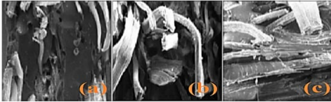
Figure 12. (a–c) SEM images of the flexural fractured specimen at different fiber loading, (a) 25 wt. %, (b) 35 wt. %, and (c) 45 wt. % of pineapple-reinforced polyester composites. Reprinted with the permission from Reference [56]. Copyright 2019 Elsevier.
