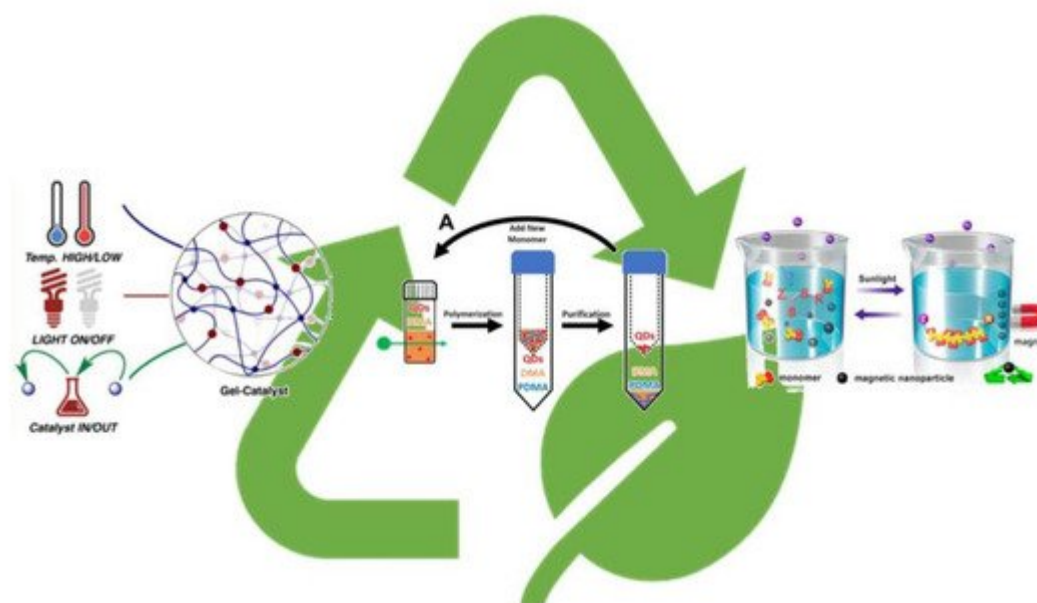
Figure 7. Recyclability of photoredox catalyst in PET-RAFT process. Adapted from refs. [27][28][29].
