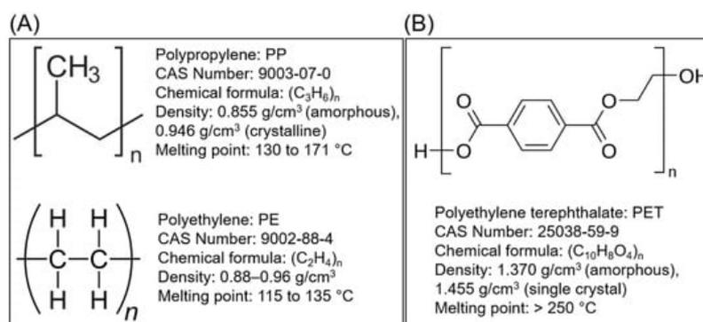
**Figure 1.** Structural and physicochemical characteristics; (A) category of non-hydrolysable plastics examples with a C–C backbone, and (B) category of hydrolysable plastics examples with a C–O backbone.
