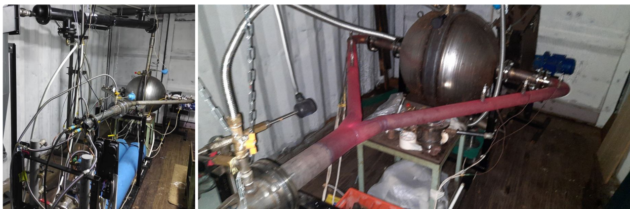
Figure 9. (a) Gasification plant based on pulsed USS gun and (b) thermal radiation of the uncooled USS gun during operation.
