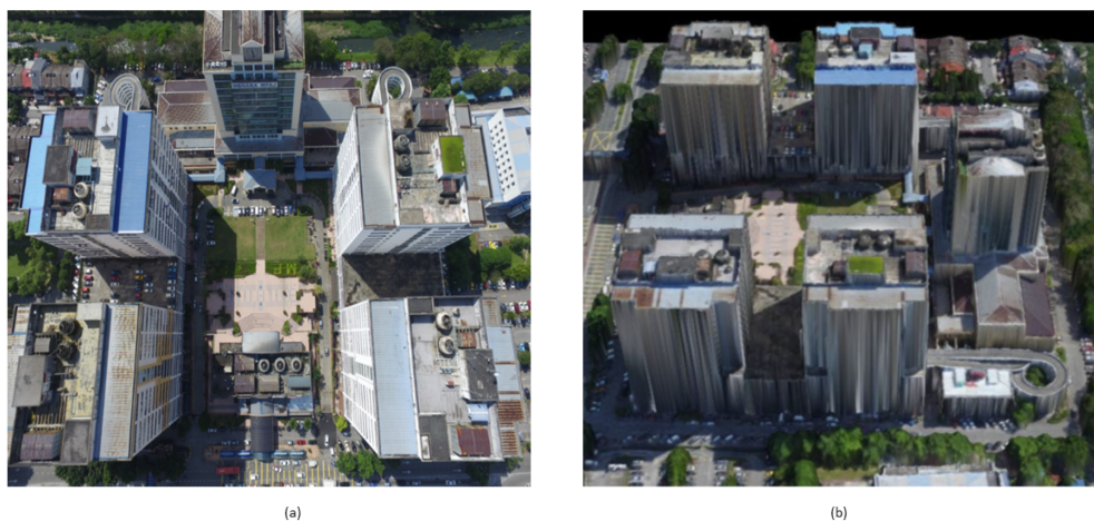
Figure 3. Type of imagery (a) 2D aerial imagery acquired via UAV; (b) 3D model built from UAV imagery.
