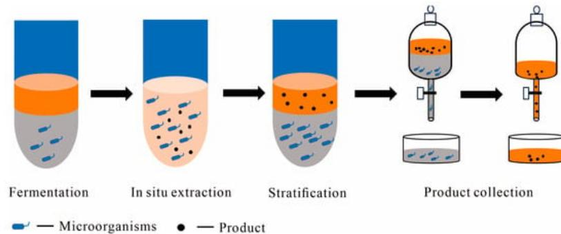
**Figure 2.** Scheme of aqueous–organic TPF and post-treatment, with main steps including fermentation, in situ extraction, post-fermentation stratification, and product collection; the orange color on the upper layer represents organic solvent or another aqueous solvent, the dark gray color on the lower layer represents the culture medium, and the light orange color of in situ extraction represents two phases mixed during the in situ extractive fermentation.
