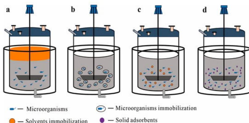
**Figure 1.** A concept of different types of TPF in a bioreactor: (a) liquid–liquid TPF systems, where the orange color on the upper layer represents organic solvents or another aqueous solvent and the dark gray color on the lower layer represents the culture medium; (b–d) different types of liquid–solid TPF systems: (b) immobilized cells as the SP; (c) immobilized solvent as the SP; (d) solid adsorbents as the SP.
