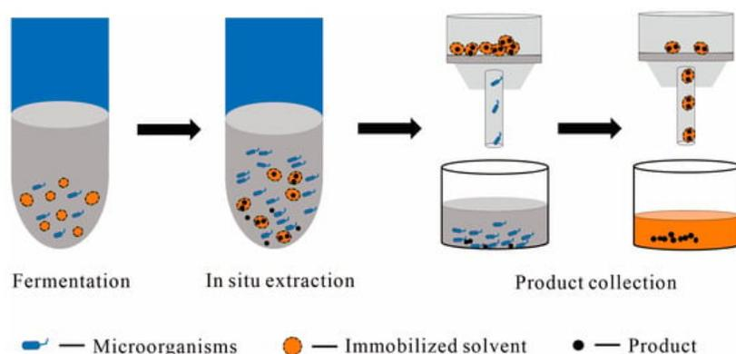
**Figure 4.** A conceptual scheme of using immobilized solvent as the solid phase in the liquid–solid TPF and downstream processing, with main steps including fermentation, in situ extraction, post-fermentation filtration, and product collection; the dark gray color represents the culture medium and the orange color represents solvents, like ILs.
