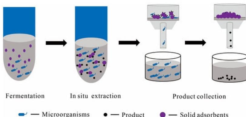
**Figure 5.** A conceptual flowchart using solid adsorbents as the solid phase in the liquid–solid TPF and downstream processing, with main steps including fermentation, in situ extraction, post-fermentation filtration, and product collection; the dark gray color represents the culture medium.
