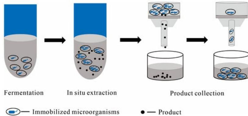
**Figure 3.** Illustration of a flowchart using immobilized cells as the solid phase in the liquid–solid TPF and downstream processing, with main steps including fermentation, in situ extraction, post-fermentation filtration, and product collection; the dark gray color represents the culture medium.
