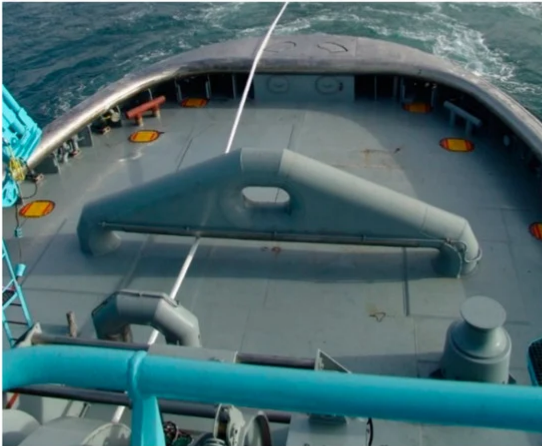
Figure 5. Wide staple of Escort Voith Water Tractor Tug “Tenax” with water spray cooling for escort towing with a high modulus polyethylene (HMPE) towline. The contact surfaces of both the staple and all around the cap rail are made of a highly polished stainless steel. Photo: Authors.
