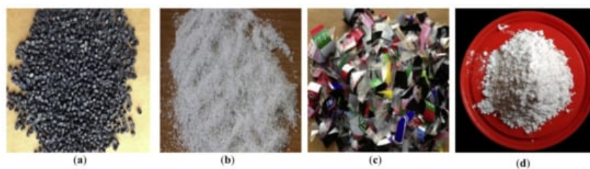
Figure 1. Various forms of waste plastics used as modifiers: (a) pellet [9]; (b) shredding [4]; (c) flake [9]; (d) powder [10]. Reprinted with permission from Refs. [4][9][10]. Copyright 2014 Elsevier publisher.
