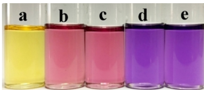
Fig. 7. Colorimetric study of the receptor ( 2.5 \times 10^{-5} M) in DMSO upon the addition of various concentrations of F^- in TBA salt form (a) receptor R1, (b) 1 equiv., (c) 5 equiv., (d) 10 equiv., (e) 50 equiv.
