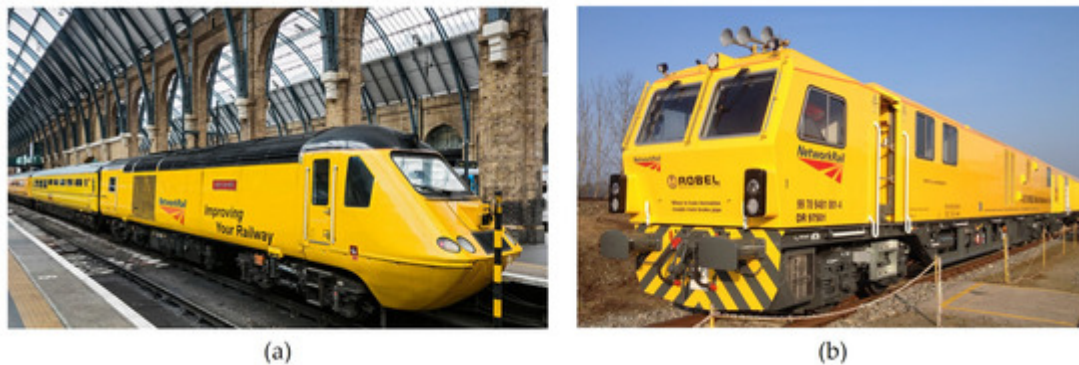
Figure 3. Specially designed train in the UK for railway maintenance: (a) new measurement train (NMT) [30]; (b) mobile maintenance train (MMT) [31].
