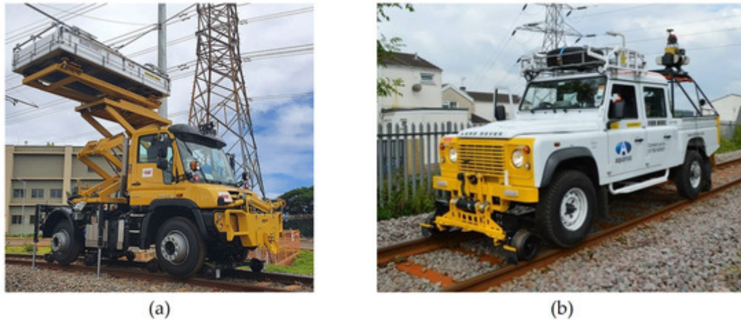
Figure 2. Road–rail vehicles for track maintenance: (a) Unimog road rail vehicle for overhead line maintenance [24]; (b) mobile asset management RRV [23].
