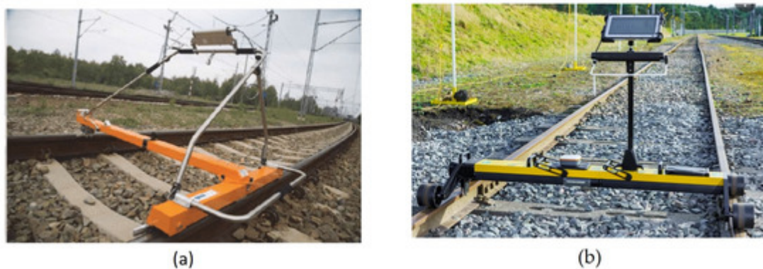
Figure 1. Track geometry inspection trolley: (a) track geometry validation trolley [20]; (b) track geometry inspection trolley with GPS [21].
