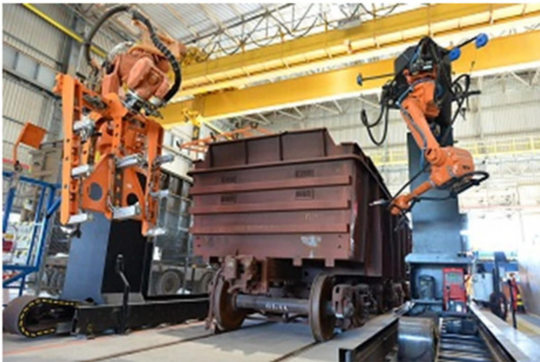
Figure 8. Robot used for repairing rail cars in mining operations [67].
