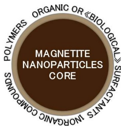
Figure 1. Schematic representation of possible surface coating of MNPs.
