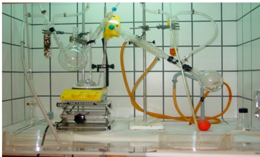
Figure 4. Installation used for the synthesis of the CZTS precursor solution at the authors' facilities.
