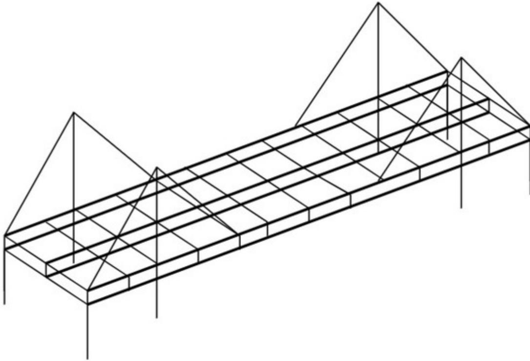
**Figure 4.** Multi-scale model with deck plate elements.
