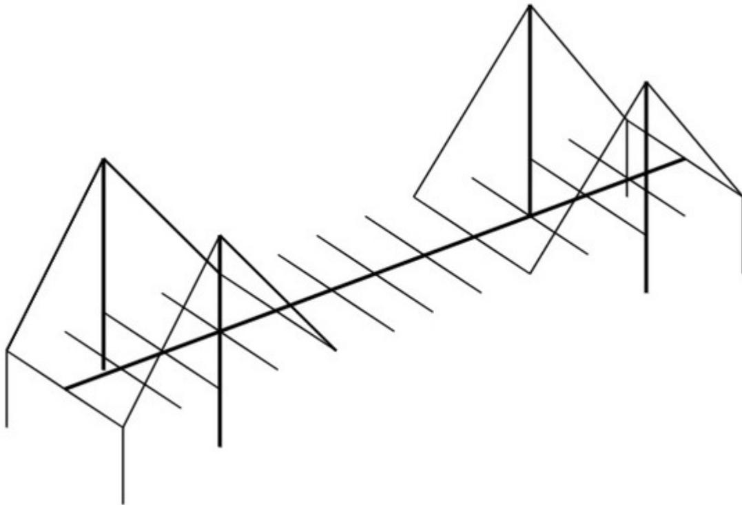
**Figure 1.** Spine-beam or single-girder model.
