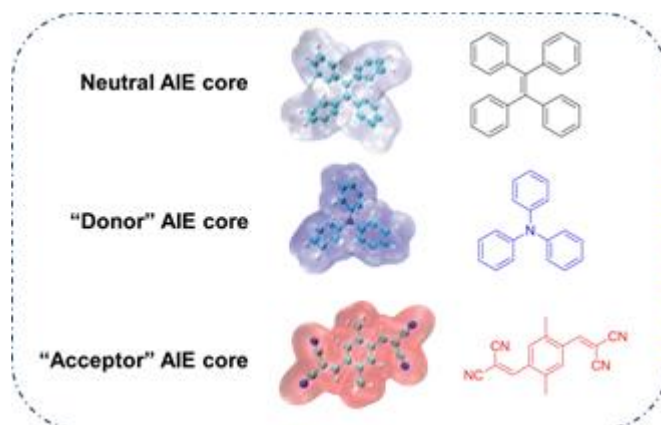
Figure 5. Classification of neutral, donor and acceptor AIE cores by their electron characters, the electronic clouds are represented by colored clouds (the neutral, donor and acceptor AIE cores are represented by the black, blue and red scheme, respectively).
