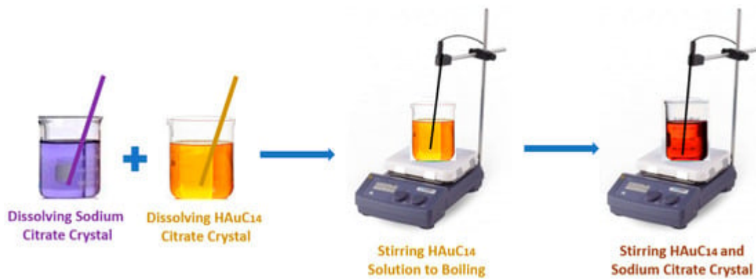
Figure 1. Gold nanofluids synthesis method based on citrate crystal dissolution.
