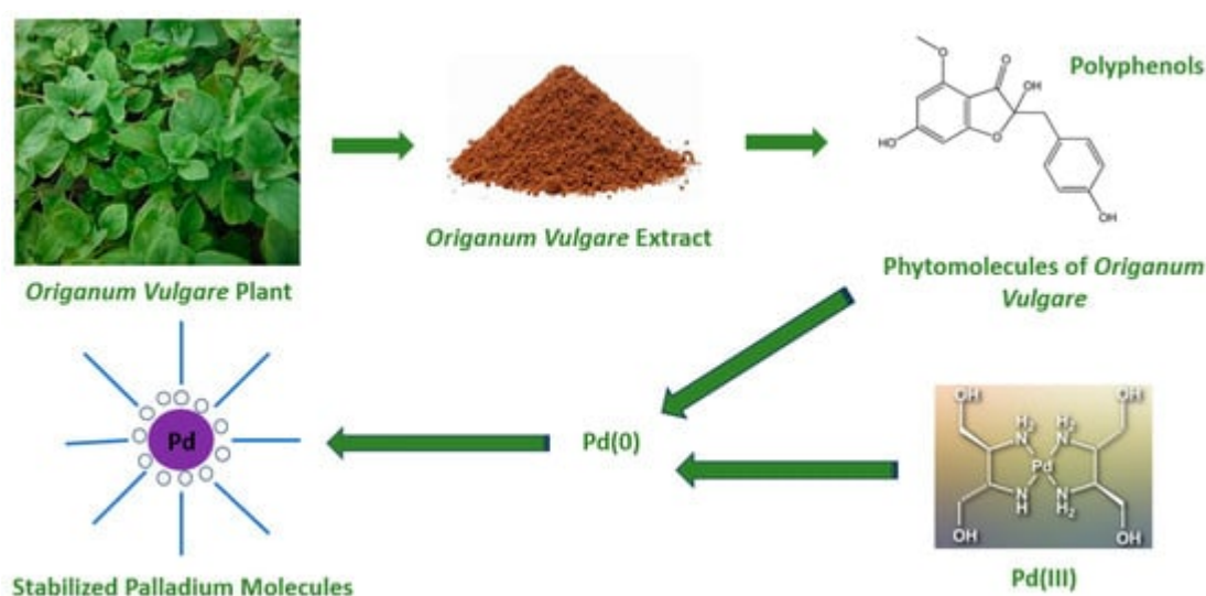
Figure 8. Typical green preparation method to synthesize palladium nanoparticles from Origanum vulgare plant.
