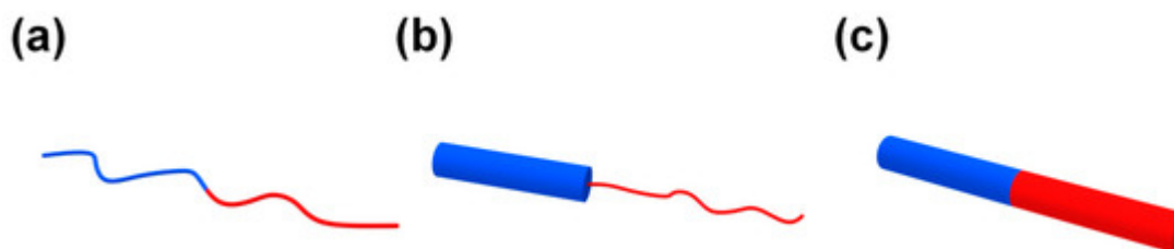
Figure 3. (a) Conventional "coil-coil" block copolymers (BCPs); (b) "rod-coil" conjugated block copolymers (cBCPs); and (c) "rod-rod" cBCPs.
