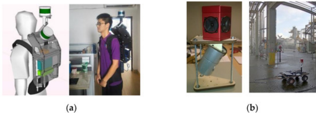
Figure 11. A push-broom 3D LiDAR. (a) The prototype in [16][17][18]; (b) left: the prototype in [19], in which the red device mounted above is a ladybug panoramic camera, it is used to perceive colors. The silver-white device mounted obliquely below is a 32-line 3D LiDAR Velodyne HDL-32e; right: the prototype is carried by a trolley.
