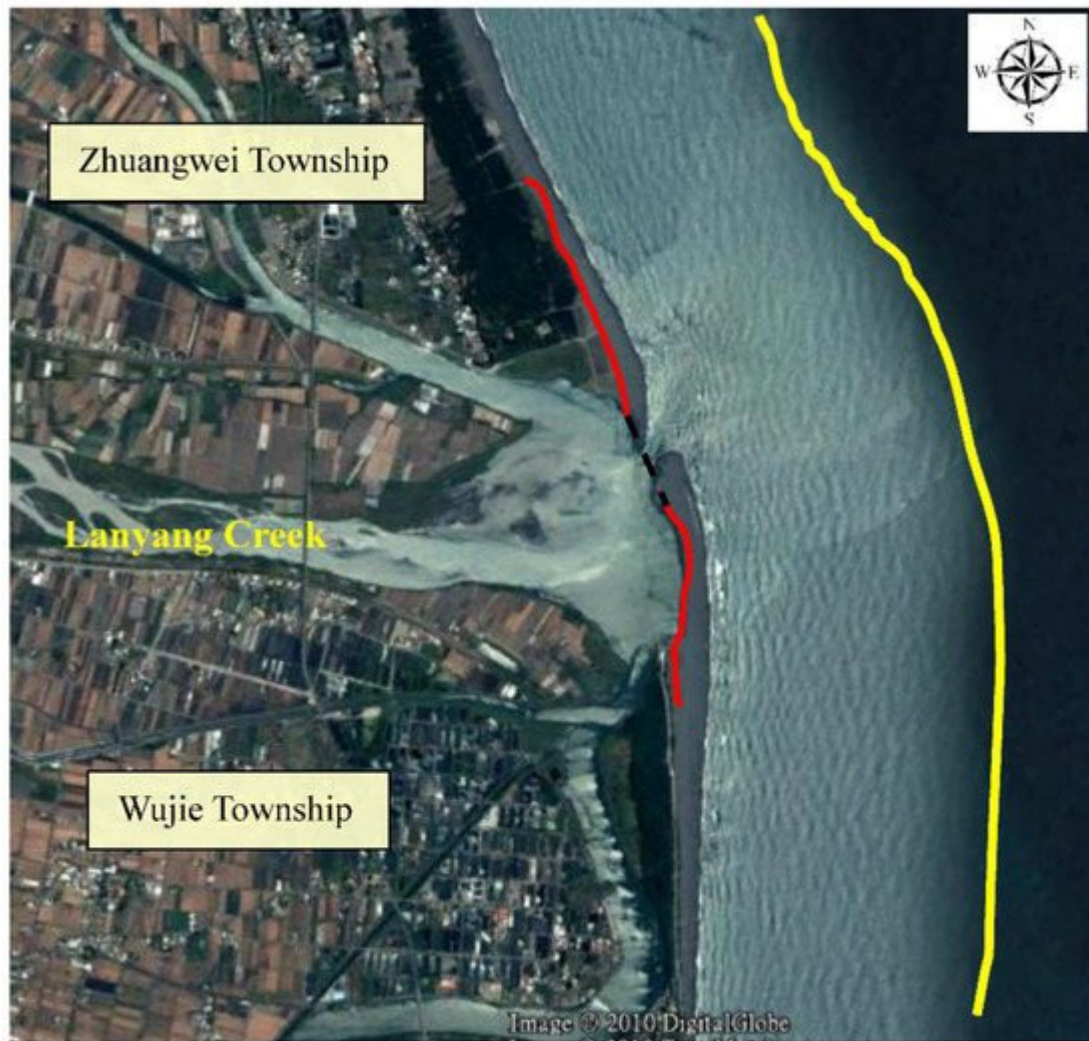
Figure 8. Preliminary planning results of coastal buffer zone using the SBEACH and wave run-up models (the estuary of Lanyang Creek, Yilan, Taiwan) [41] . (Red line: the onshore boundary of the coastal buffer zone; yellow line: the offshore boundary of the coastal buffer zone.).
