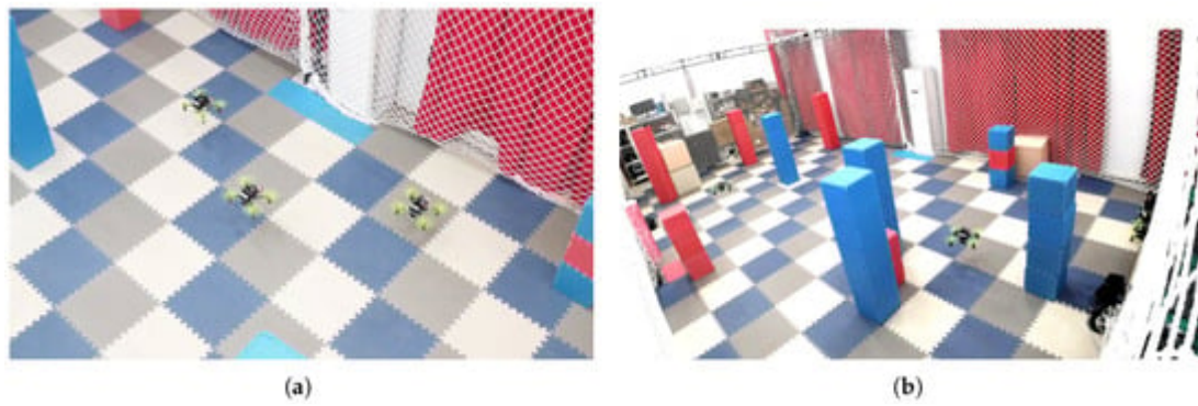
Figure 1. The practical experiments. (a) shows the initial status of three UAVs; they are placed on the same side of a room. (b) shows three UAVs are performing exploration in one trial; a 10 \times 8 \times 3 m virtual boundary is set to bound the exploring space.
