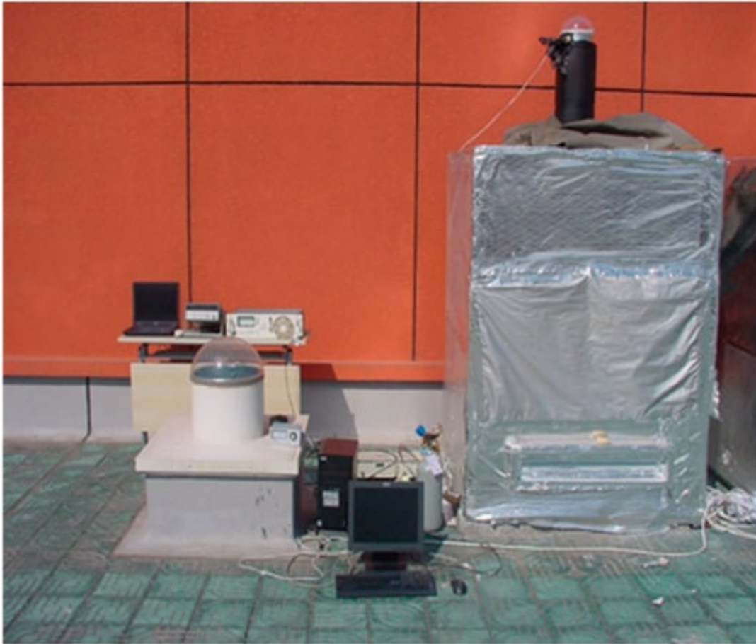
Figure 2. Light pipe-natural ventilation system experimental apparatus.
