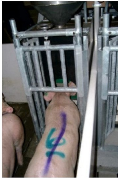
Figure 1. IVOG—A station for individual feed intake recording in group housing (Instentec B.V., Marknesse, the Netherlands) used in the studies of De Haer and Merks, [21] , De Haer et al. [36] , De Haer and de Vries, [37] , Georgsson and Svendsen, [38][39] , Rauw et al. [40] , and Fernández et al. [14] .
