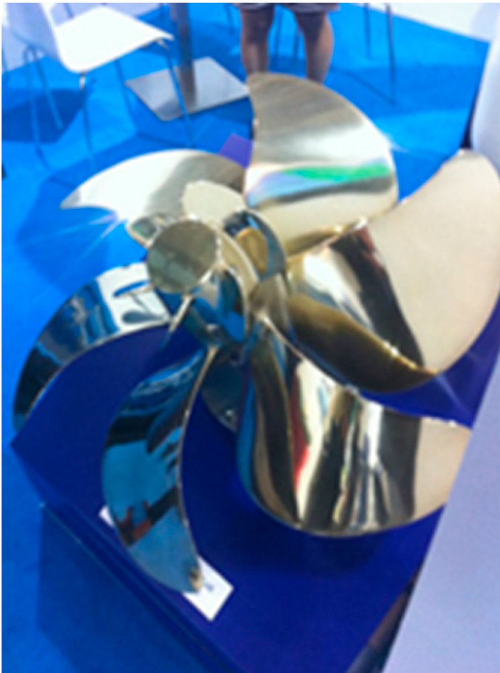
Figure 3. Post-swirl devices: PBCF [5] .
