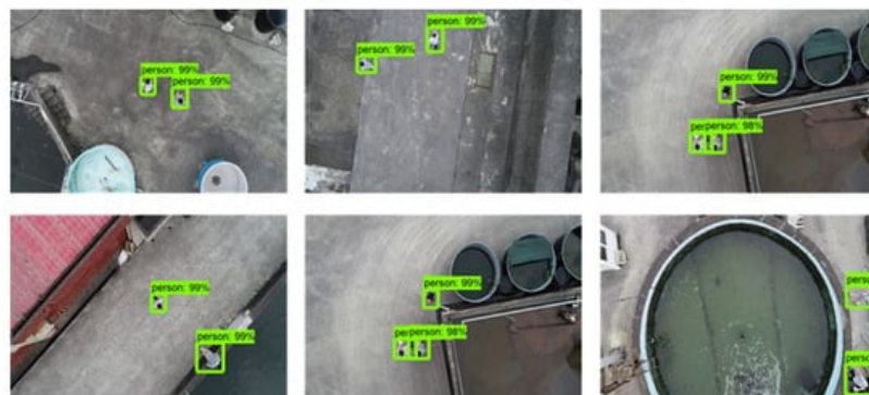
Figure 16. The results of the person detection and recognition.
