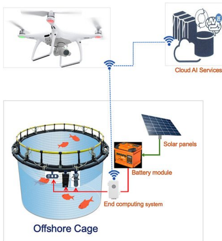
Figure 19. Drone as WIFI communication channel from offshore cages to cloud AI services.
