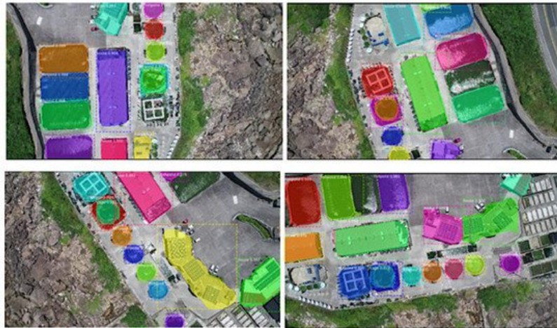
Figure 12. The results of semantic object detection.
