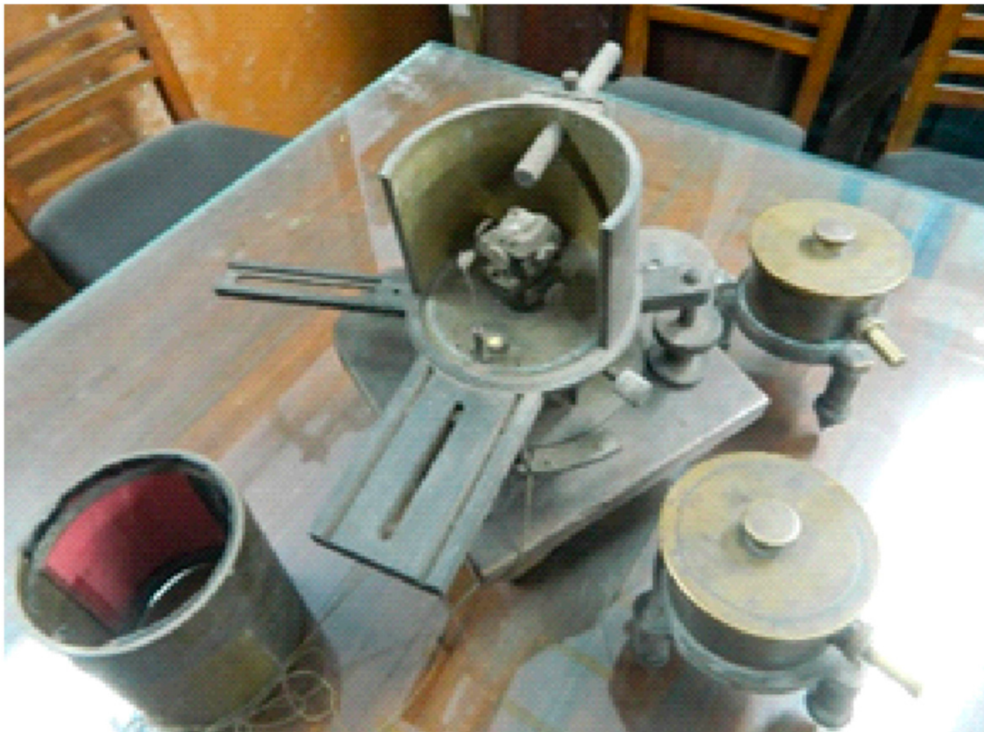
Figure 4. X-ray Diffraction Apparatus built by SN Bose. (Courtesy: Prof. Alok Mukherjee).
