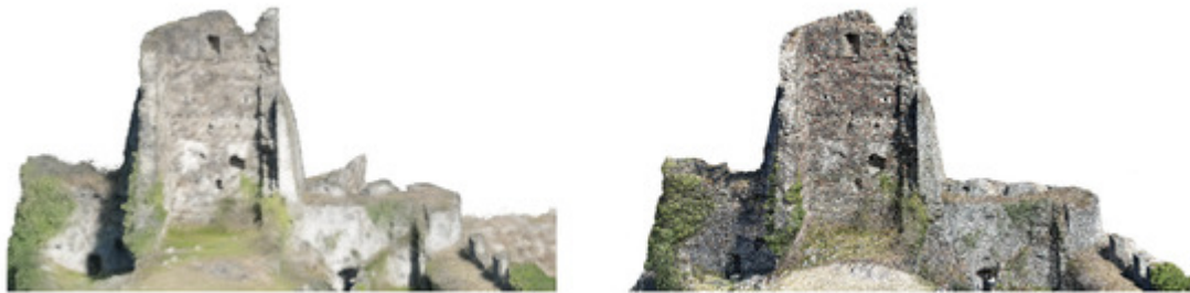
Figure 4. Point clouds produced with Nerfstudio ( left ) and Metashape ( right ) using the same set of images for the Vogogna dataset.
