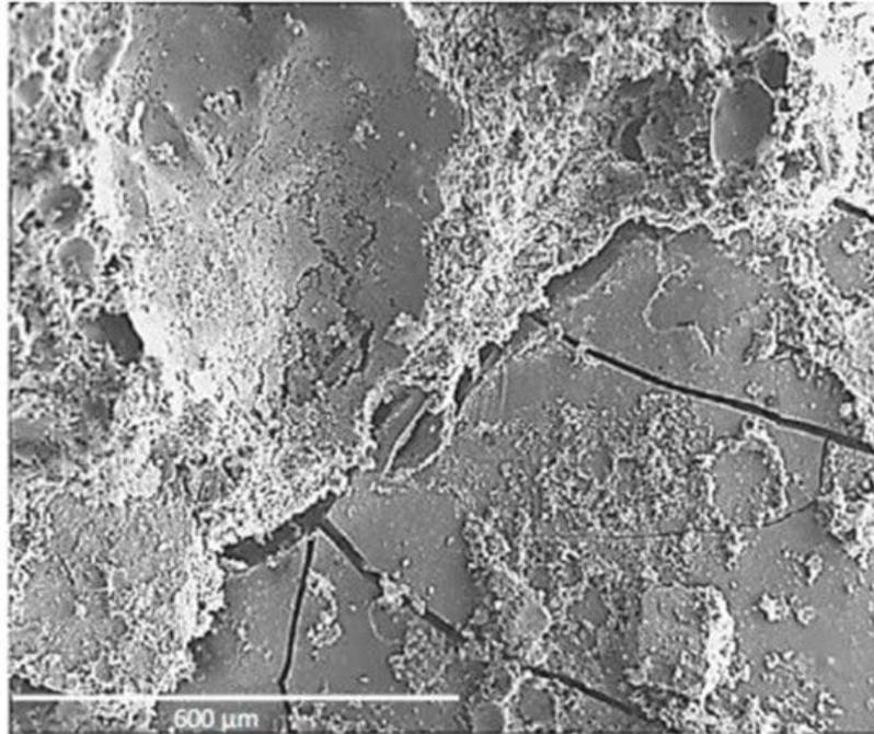
**Figure 4.** Cracks in seashell particles and cement paste [33].
