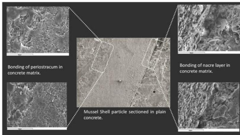
**Figure 3.** SEM observation of microstructure of seashell concrete [8].
