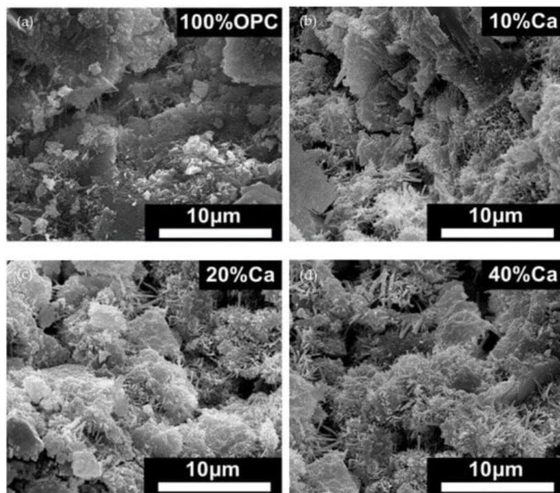
**Figure 5.** SEM of hydrated cement matrix produced in seashell cement mixtures <sup>[10]</sup>: (a) 100% OPC; (b) 10%Ca mixture; (c) 20%Ca mixture; (d) 40%Ca mixture.
