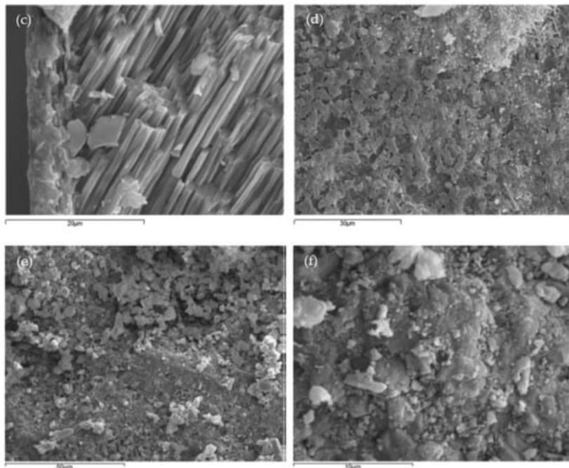
**Figure 1.** SEM analysis of mussel shell composition by Martínez-García et al. [32]: (a) periostracum (external layer)—prismatic structure layer; (b) periostracum layer front view; (c) prismatic structure layer; (d) nacre layer front view; (e) nacre layer; (f) limestone particle.
