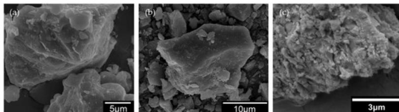
**Figure 2.** Particle surface morphology of (a) limestone powder; (b) Portland cement powder; (c) seashell powder [10].
