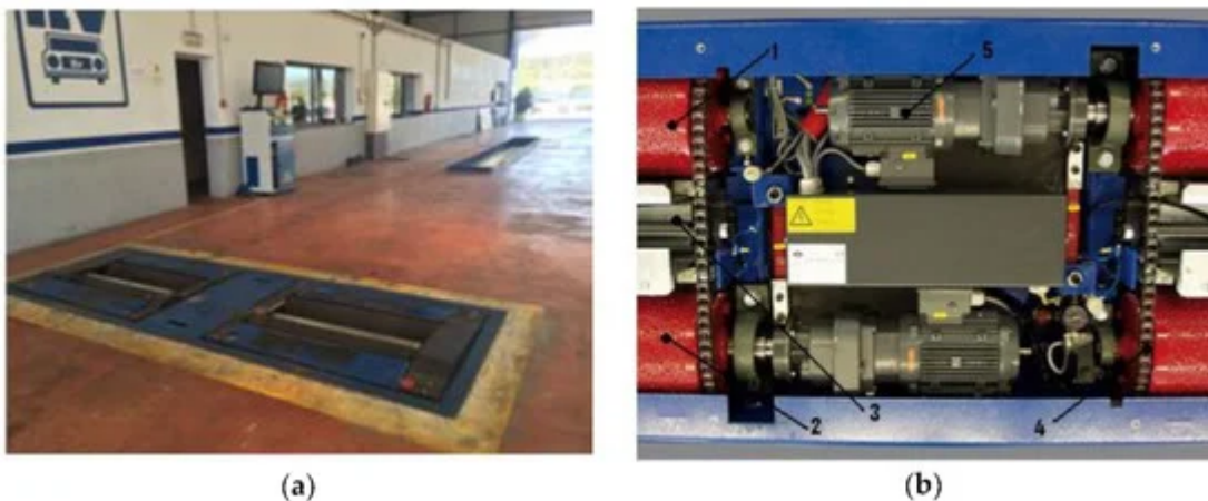
Figure 1. Roller brake tester. (a) General view and (b) main elements.
