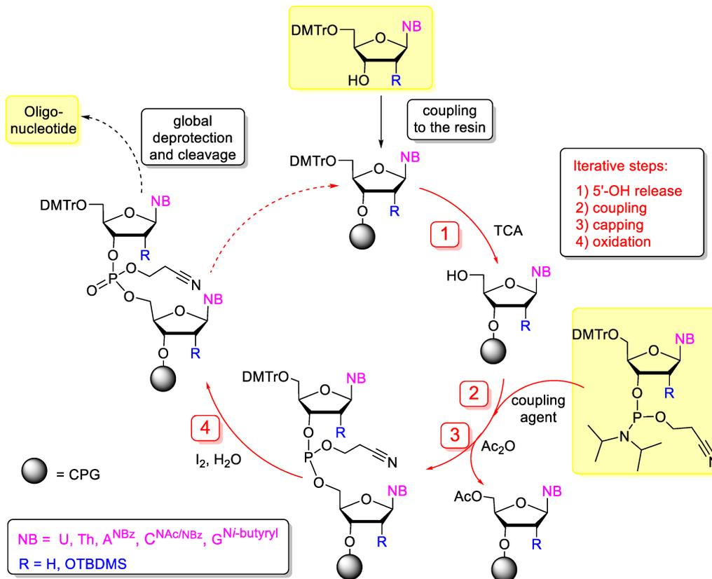
**Scheme 1.** Solid-phase synthesis of oligonucleotides by phosphoramidite chemistry. The iterative steps of synthetic cycle are highlighted in red. DMTr: 4,4'-dimethoxytrityl, TBDMS: *t*-butyldimethylsilyl, TCA: trichloroacetic acid, Ac<sub>2</sub>O: acetic anhydride, CPG: controlled pore glass.
