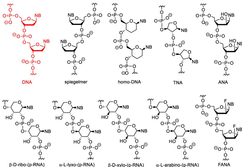
**Figure 2.** The structure of DNA and XNAs with other sugars than  $\beta$ -D-ribofuranose.
