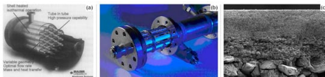
Figure 3. (a) Isothermal module concept Pervap ® SMS (silica membrane system) from Sulzer Chemtech, adapted from [16], with permission from Copyright (2004), Elsevier Science B.V. (b) Bench-scale seven membrane shell-and-tube design module with baffles and perpendicular feed flow, adapted from [17], with permission from Copyright (2005), Elsevier Ltd. (c) SEM cross-section of an amorphous silica membrane (scale 1:500), adapted from [18] with permission from Copyright (2005), Elsevier B.V.
