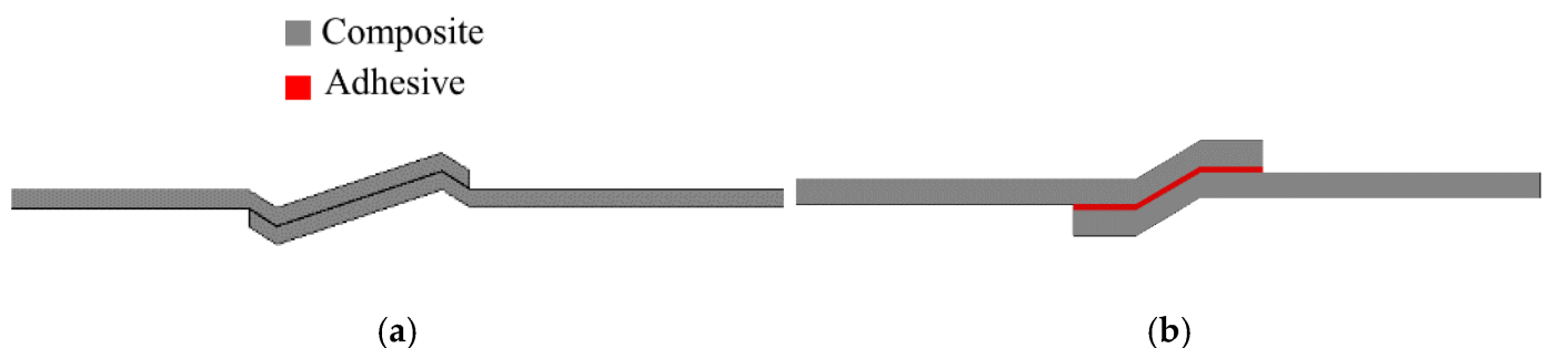
Figure 5. (a) Wavy-lap joint and (b) flat joggle flat joint (FJF).
