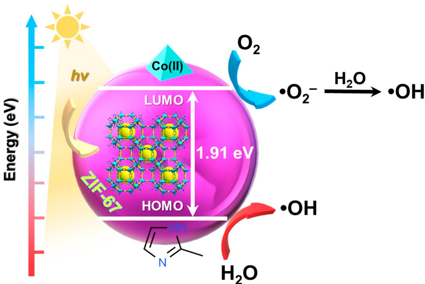
**Figure 1.** Scheme representing the photodegradation reaction mechanism involving ZIF-67.
