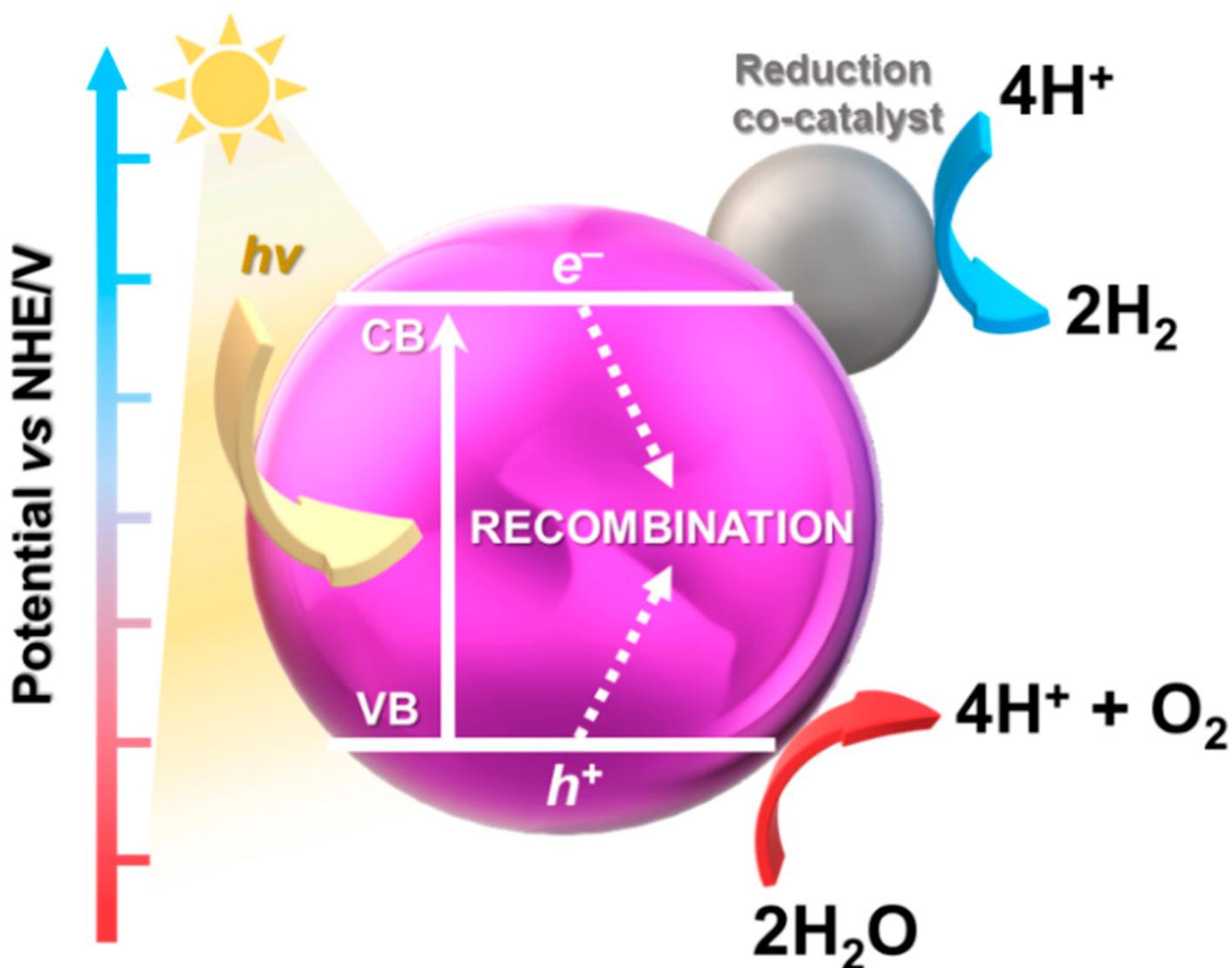
Figure 2. Scheme of light-triggered water splitting over a semiconductor photocatalyst.
