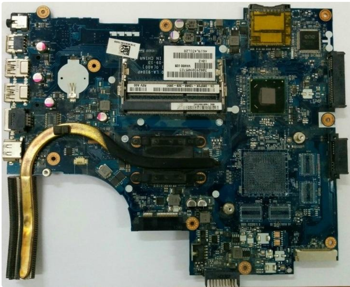
(a) hp ® motherboard with thermal management system (heat pipe).
