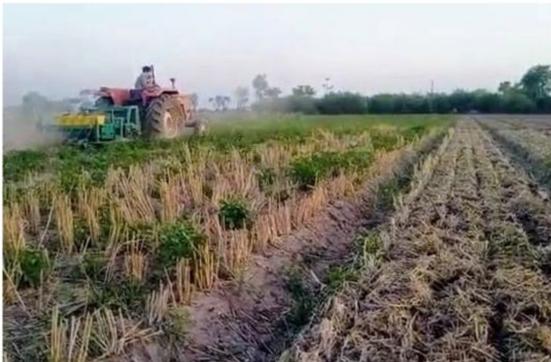
Figure 1. Mechanized no-till DSR in Pakistan, on mulched raised beds with the PQNK system. Source: Pedaver Pvt. Ltd.
